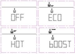
This icon will flash until the predetermined water temperature is reached.
