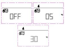
Flame icon = room temperature heating start, this icon will flash until the predetermined room temperature is reached.
