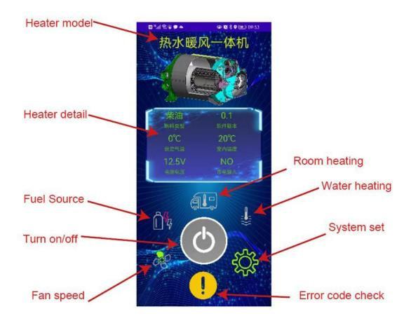
The display interface after the controller connected Bluetooth
