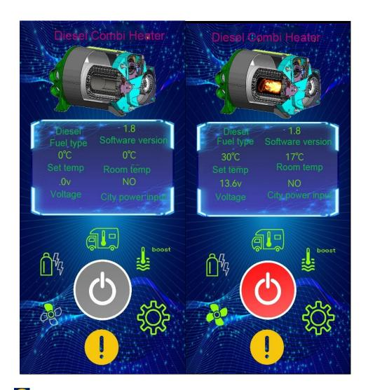
Click Perfor code button, enter the error code check and error code eliminate interface, refer below.
