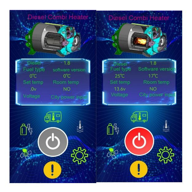
Set the room temperature, enter the number from 5-35 degrees, press OK, the setting is done.
